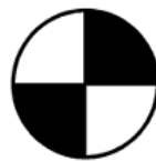
Figure 2.1 – Center of Gravity Symbol
